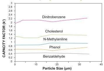
Uniform capacity (k') and selectivity (k') factors across all particle sizes for predictable and reliable scale-up
