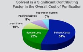
With 35Å Davisil® media, solvent consumption can be substantially reduced compared to 60Å media (~50%). Switching to a small-pore 35Å high-surface area media can be a simple way to help comply with environmental, increased productivity, and cost-reduction initiatives.
