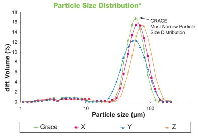
Tight particle size distribution optimizes efficiency and pressure drop in packed columns.
